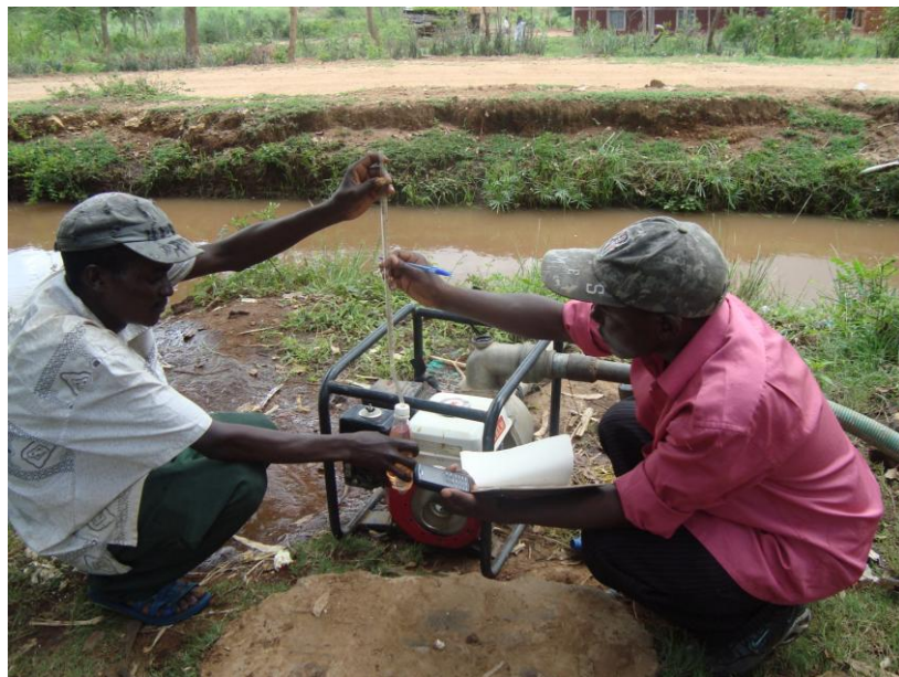
Plate 3.4. A pipette being used in fuel use determination.
