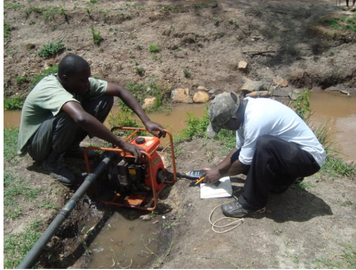
Plate 3.3. Measurement of pump speed using a hand held tachometer.
