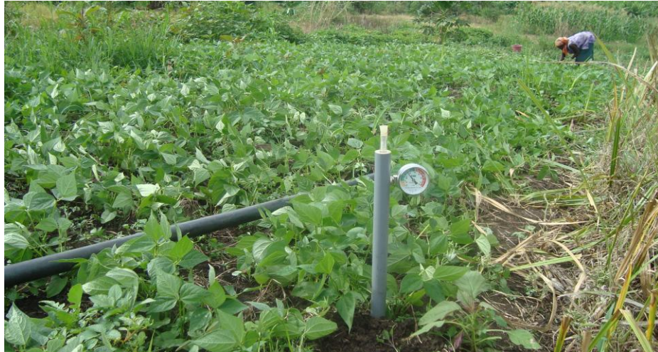
Plate 3.7. Tensiometer measures soil water tension in a French bean plantation.
