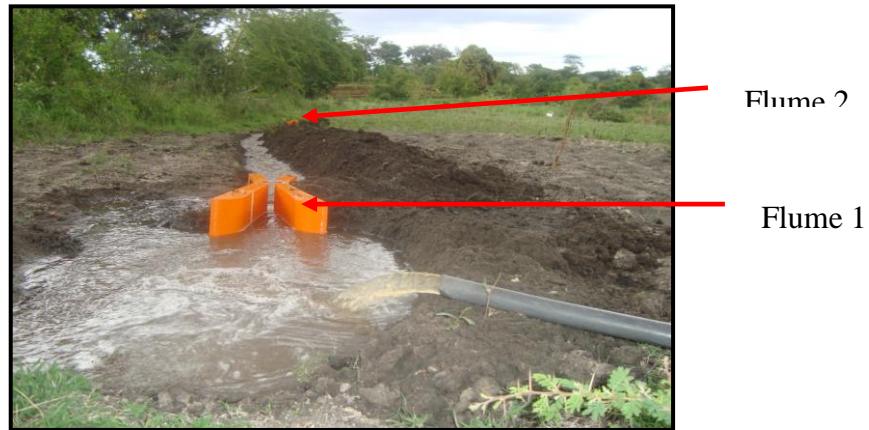
Plate 3.6. Water flow measurement using Parshall flumes in a canal.
