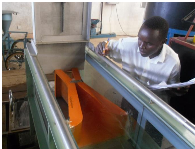
Plate 3.5. Calibration process for the Parshall flume.
