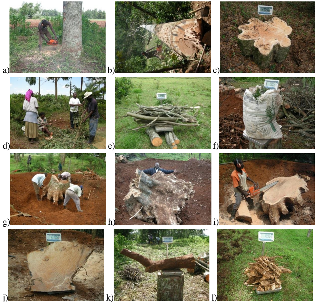
Appendix 2.1 Schematic representation of field events: (a) cutting a standing tree using a chain saw, (b) sectioning the stem, (c) weighing a sectioned stem piece, (d) stripped leaves from branches, (e) weighing branches, (f) weighing leaves, (g) excavating the root system, (h) unearthed stump (i) splitting a large stump (j) weighing a sectioned stump (k), weighing a large root (l) weighing small root pieces.
