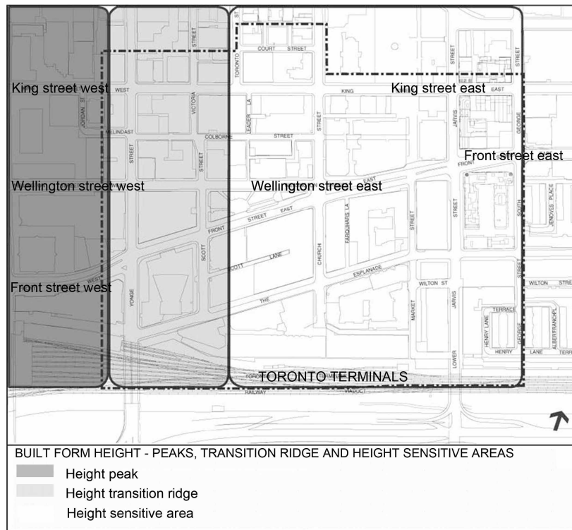
Fig. 8.15: Transition of building height from Peak area - Transition Ridge - low rise area, from http://www.toronto.ca/planning/urbd esign/st_lawrence.htm on 1 Sept. 2010.
