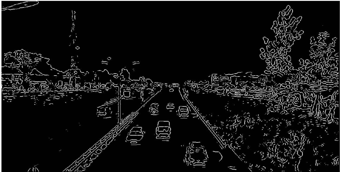
(b) Segmented frame with shadows removed
