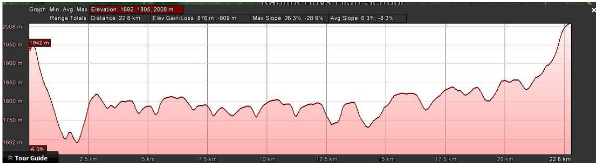
Fig. 3. Terrain profile of nodes E & F, a 24.3KM link, between Aberdare country club and Kiangwaci, Othaya, Nyeri, Kenya
