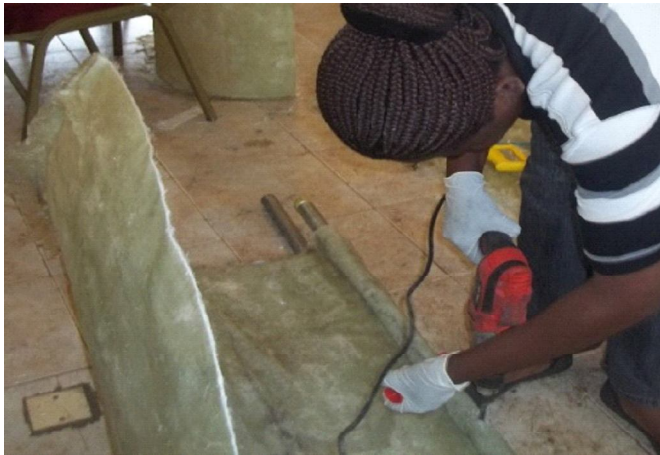
Fig. 5. The blade being drilled and joined to the live shaft using bolts
