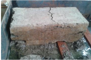
Fig. 1. Water absorption test of the blocks
