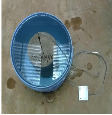
Plate 1.1: Recording of internal concrete temperature
