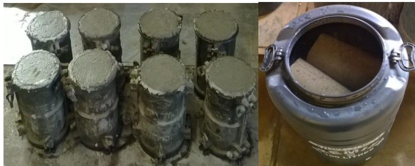
Plate 3.1: Cylindrical concrete specimens for compressive and splitting tensile strength testing
