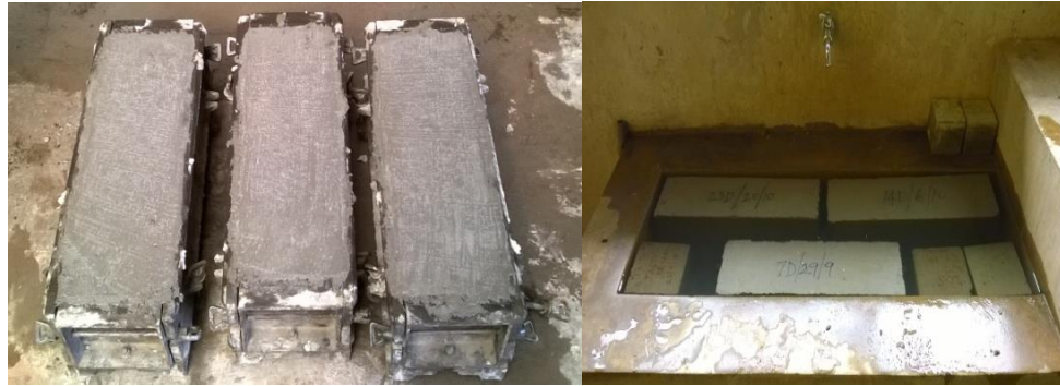
Plate 3.2: Concrete beam specimens for flexural strength testing
