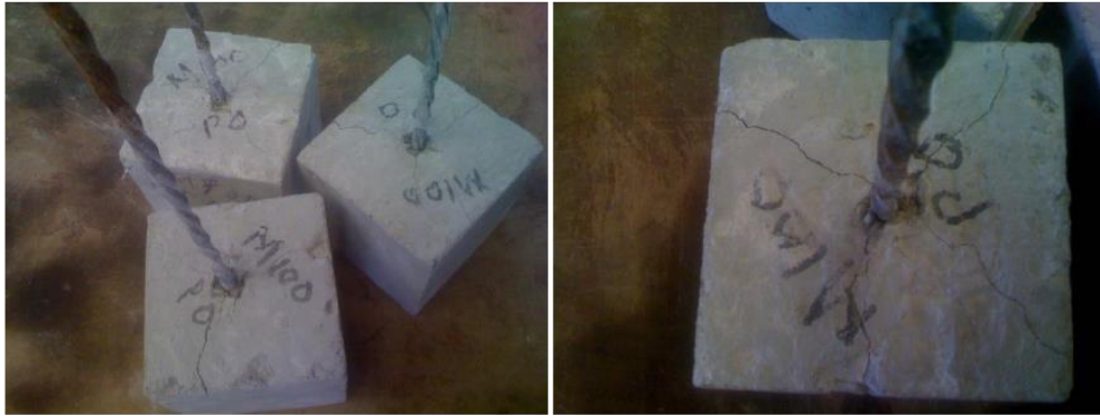
Plate 4.5: Illustration of pull out test specimens after failure
