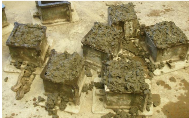
(i). Concrete cubes the preparation
