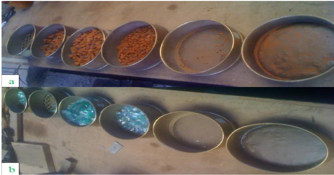
(v). Test results of test samples (clay brick aggregates and plastic fibres) after sieve analysis test.
