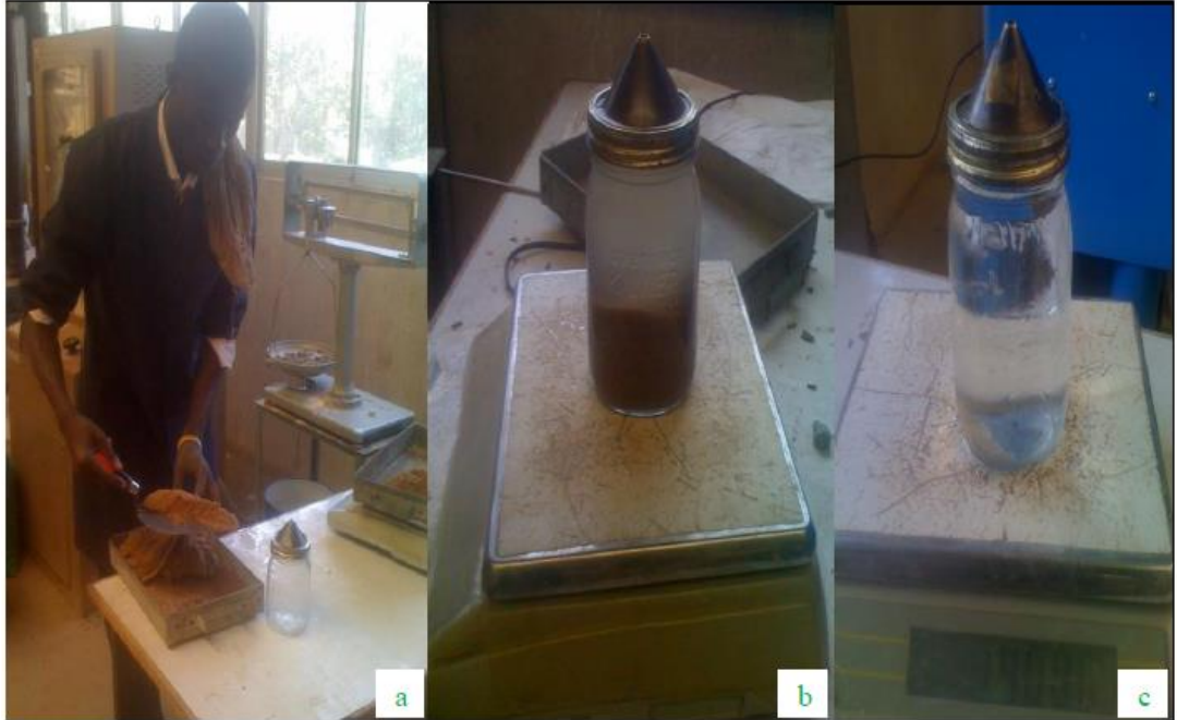
(iii). Procedure to determining water absorption and specific density of fine aggregates
