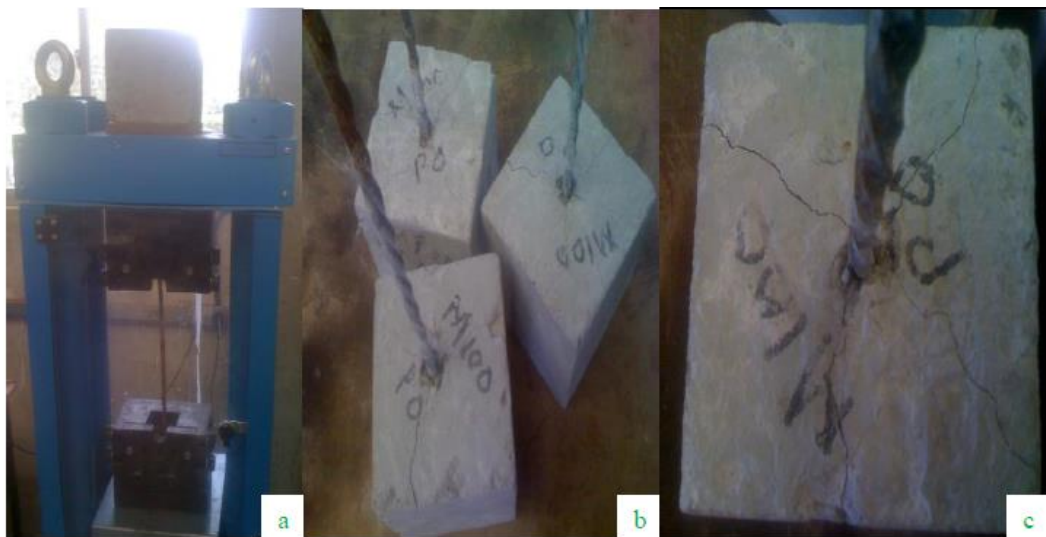
(iii). Pullout system setup, tested samples and typical failure mode
