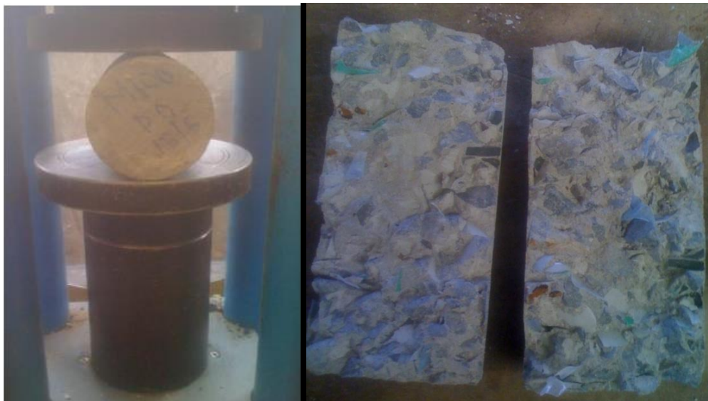
Plate 4.2: Splitting tensile sample test setup and failure mode
