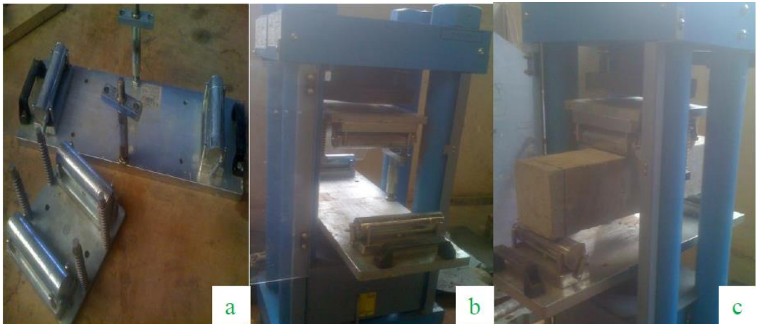
(v). Preparation for the beam support setup before test
