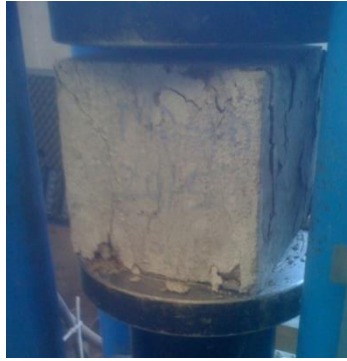
Plate 4.1: Failure of concrete cube tested for compressive strength
