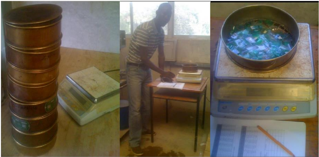
(iv). Sieve analysis test for the test samples (clay bricks aggregates and plastic fibres)
