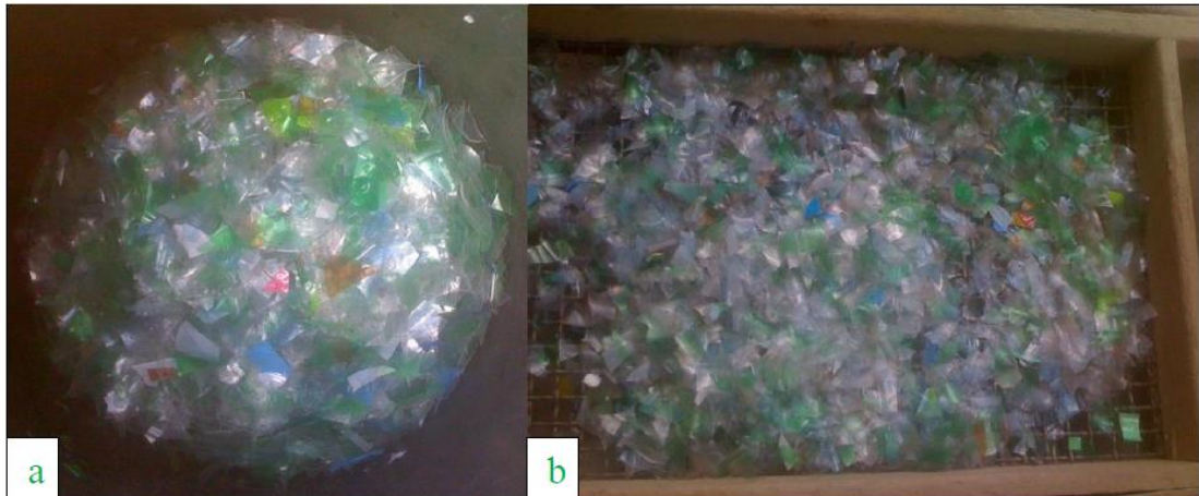
(vi). Preparation of plastic fibres to achieve size between 4.75-19mm to be used in this study
