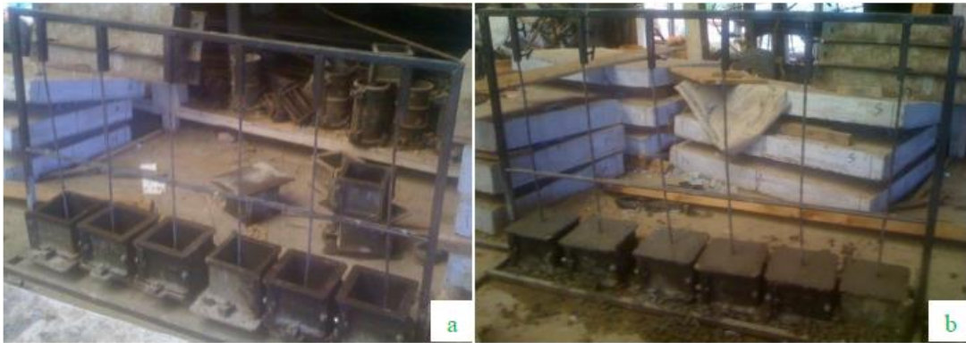
(ii). Pullout samples preparation
