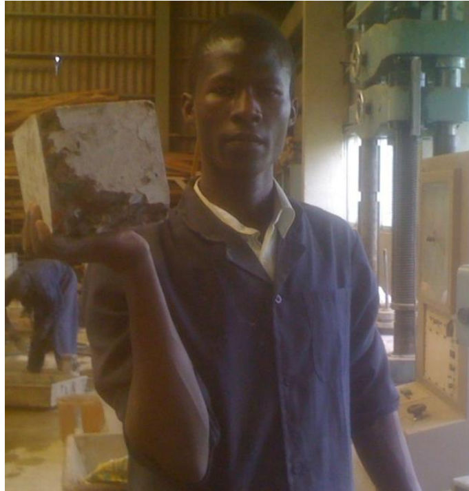
(vii). Concrete cube with plastic fibres and clay bricks aggregates after failure
