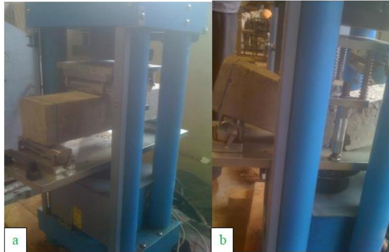
Plate 4.3: Set up of flexure beam and final failure under flexural strength.
