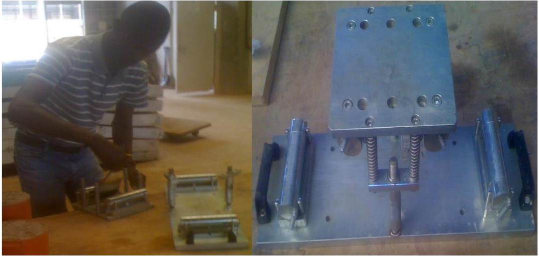
(iv). Preparation for the beam support setup before flexure test
