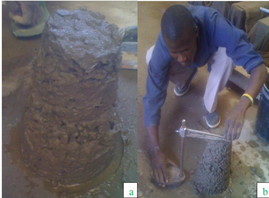
Plate 3.7: Concrete slump measurement
