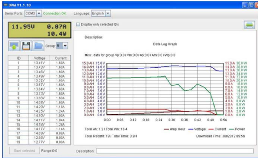
Graph 1. Data Log Graph generated by the applications software using data downloaded in GSM-SMS transmission mode
