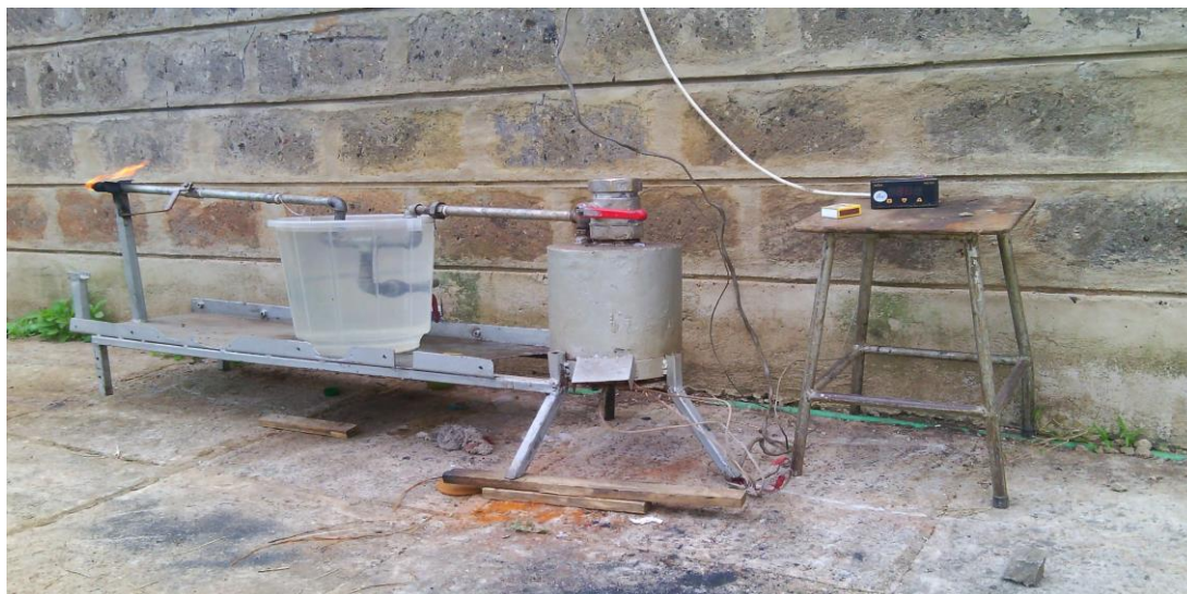
Plate 1: Pyrolysis batch reactor used for oil production
