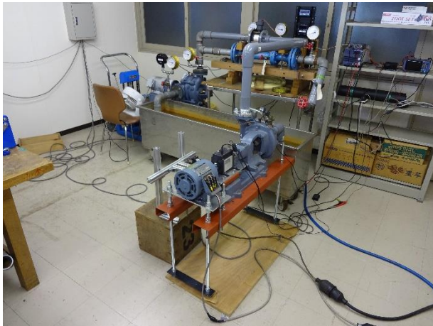
Fig. 4 Experimental apparatus for hydro turbine generator tests
