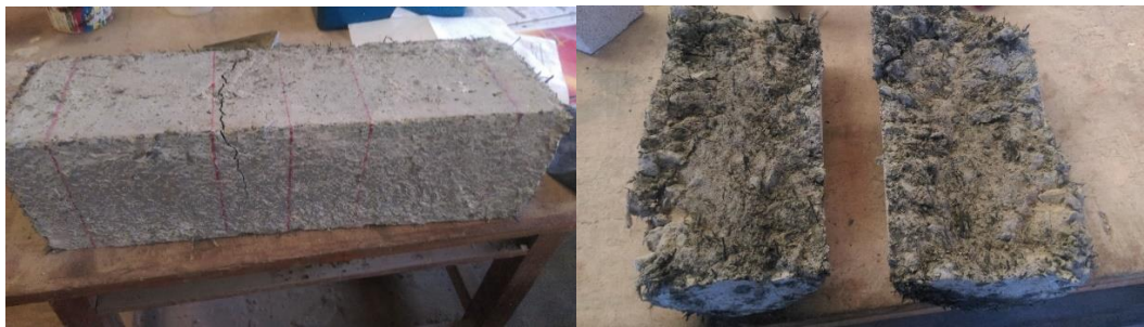
Fig. 4.16: Specimens failure pattern, (a) Beam Failure under Flexural Test (b) Splitting Tensile Strength Test
