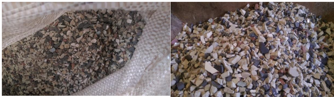
Fig. 3.2: Fine and Coarse Ceramic Tiles Aggregate
