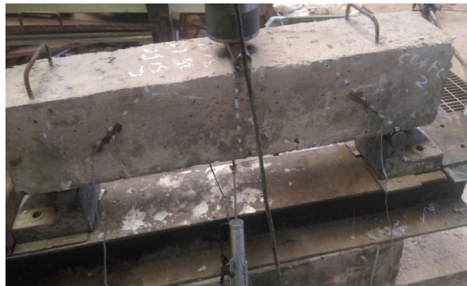
Fig. 3.5: Simple Supported Beam Subjected to Three-point Load
