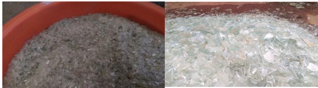
Fig. 3.3: Fine and Coarse Glass Aggregate
