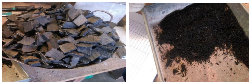
Fig. 3.4: Fine and Coarse Rubber Tyres Aggregate
