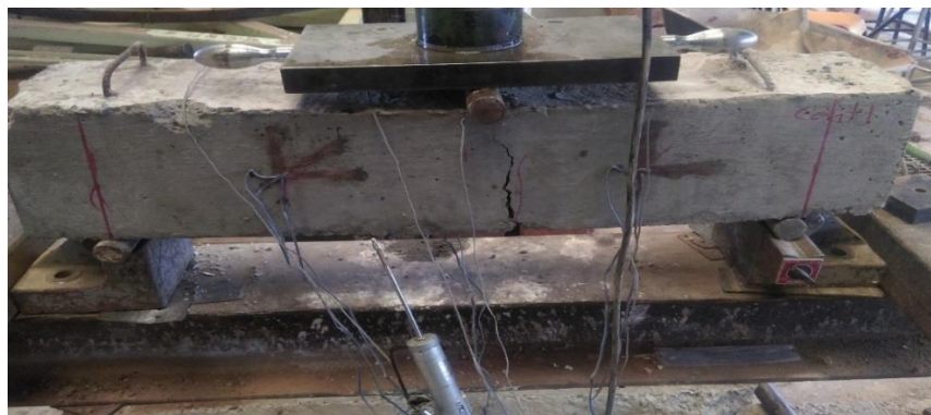
Fig. 4.17: Test of the Beam Under Three-Point Load
