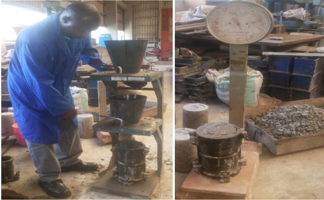
Figure 3.4: (a) Compaction factor test
