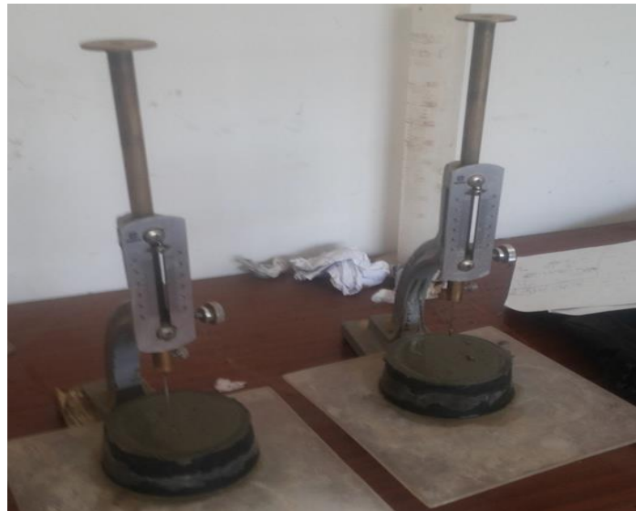
Figure 3.1: Experimental set up for consistency and setting time for blue gum ash cement
