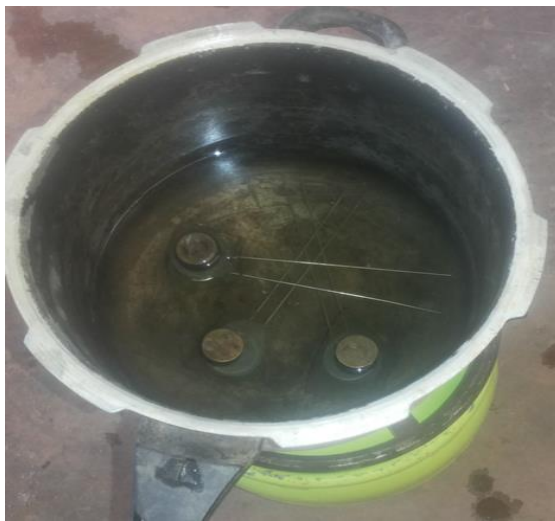
Figure 3.2: Experimental set up for soundness of blue gum ash cement
