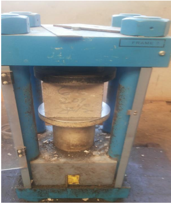
Figure 3.5: Compressive strength test
