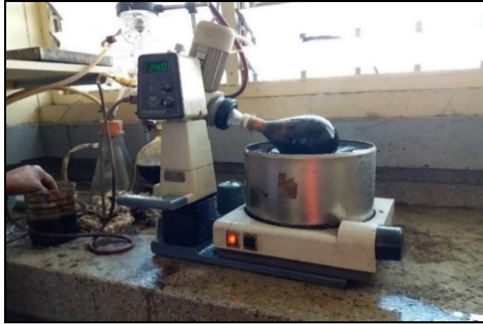
Figure 3.4: Rotary Evaporator Method
