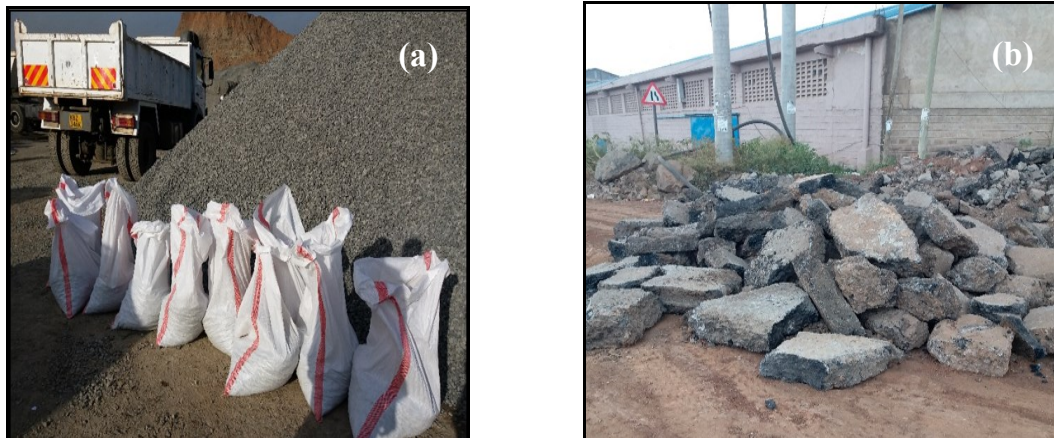
Figure 3.2: Material Collection: (a) Virgin Aggregates; (b) RAP Aggregates
