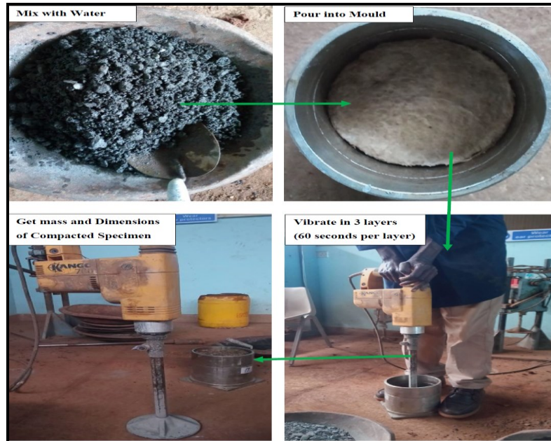
Figure 3.7: Vibrating Hammer Method
