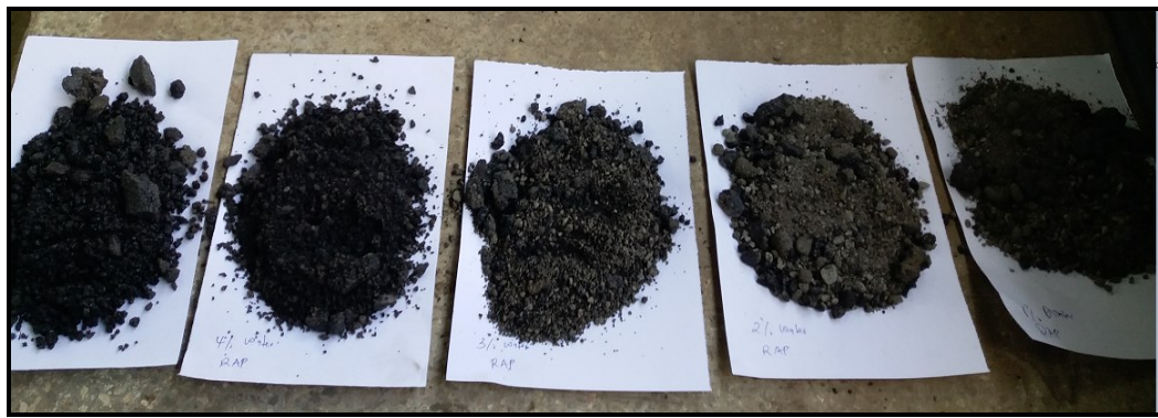
Figure 3.6: Coating test - Air curing of coated aggregates
