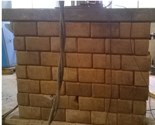
Figure 0.10: Crack propagation and wall failure mode for LSW3
