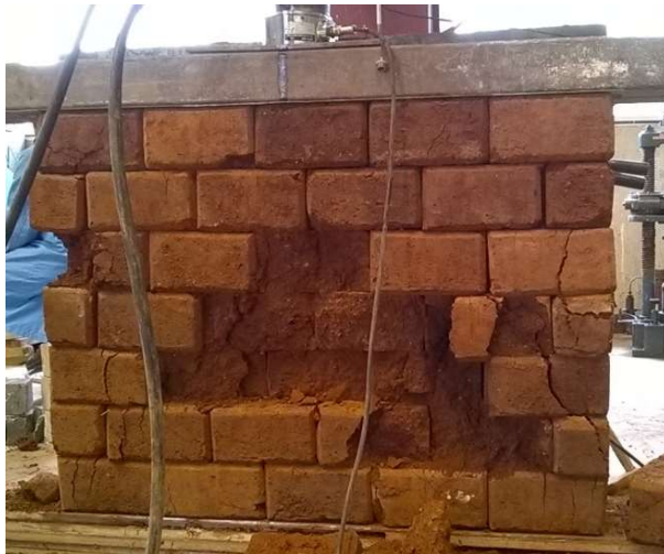
(c) CSW6 failure
