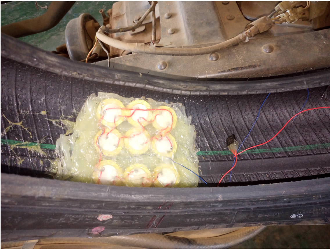
Figure 3.9: Gluing of the piezoelectric patch in the car tire
