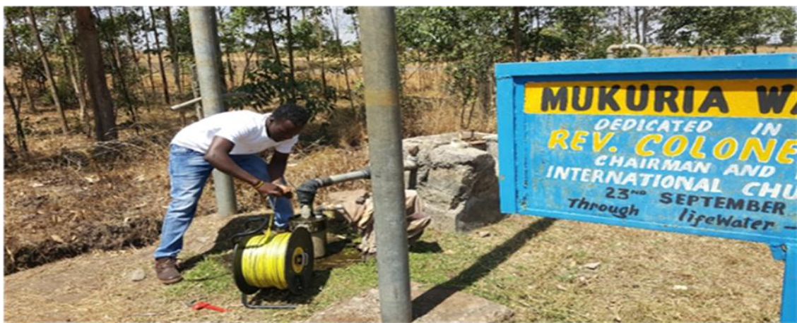
Plate 3.1: Measuring Groundwater Depth Using Dipper-T Water Level Meter
