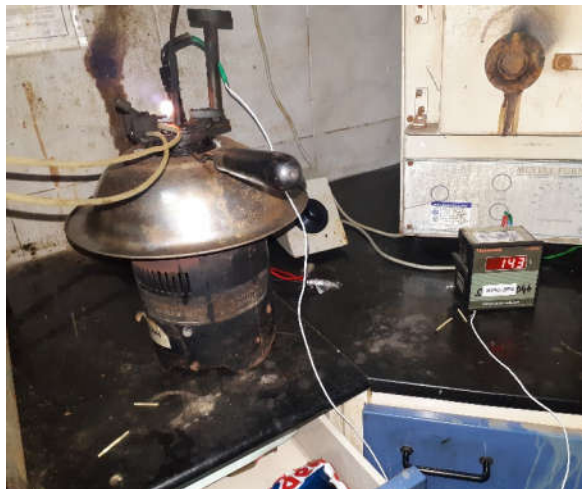
Figure 3.11: Flash Point measurement set up.
