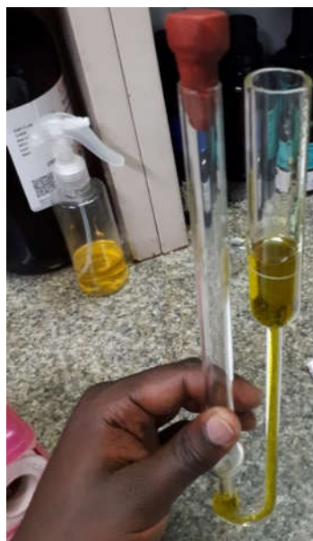
Figure 3.15: Glass capillary kinematic viscometer for measuring viscosity.
