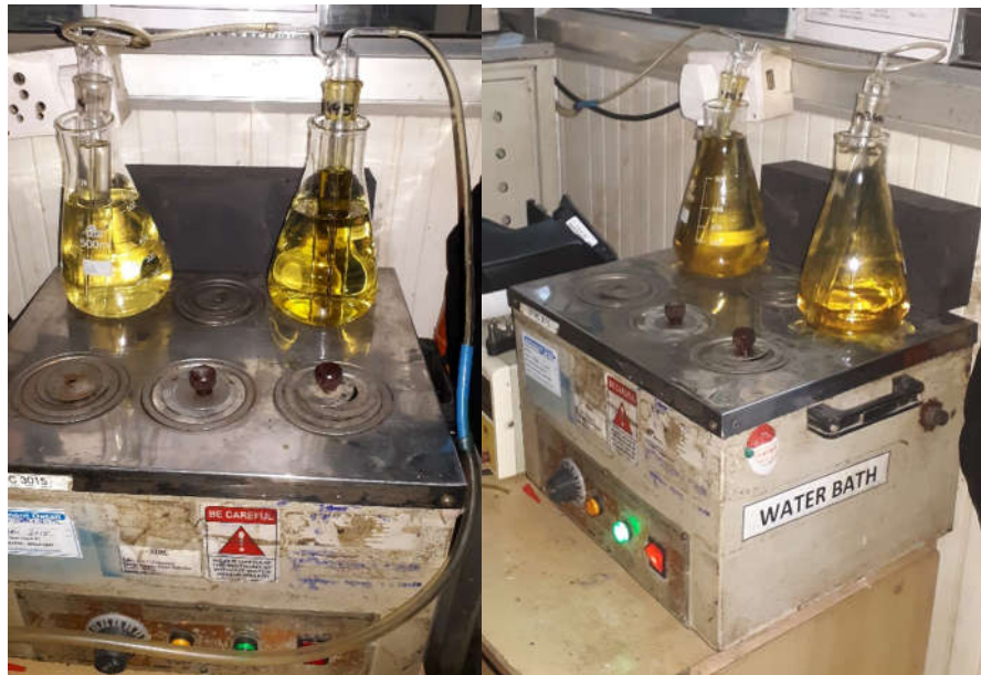
Figure 3.10: Oxidation stability measurement set up.
