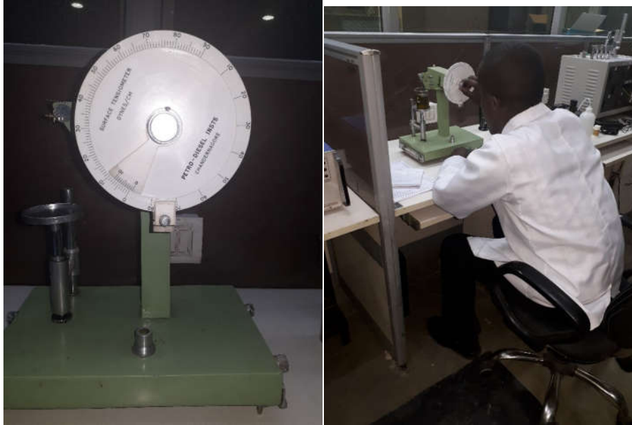
Figure 3.17: Interfacial tension set up.
