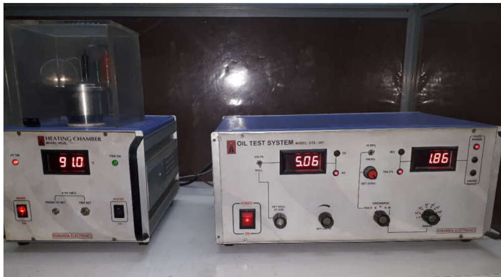
Figure 3.4: Tan-delta set up.
