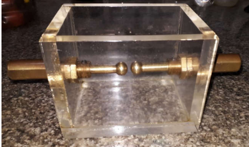
Figure 3.2: The BDV Test Cell.
