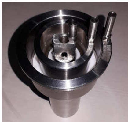
Figure 3.7: Test Cell for carrying specific resistance test.
