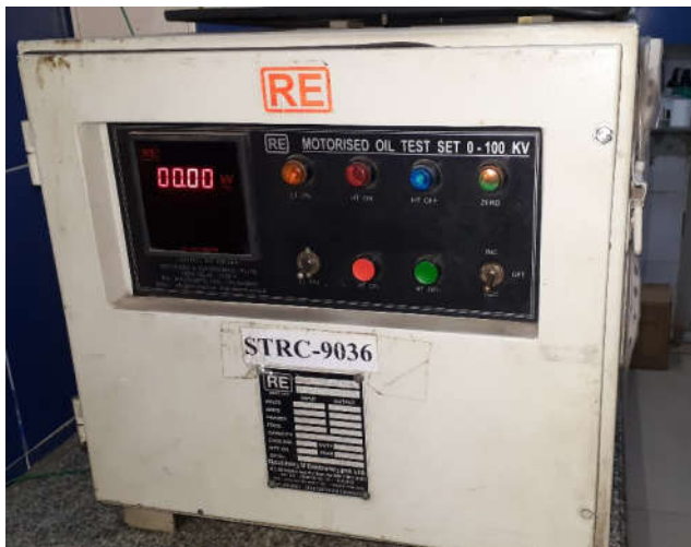
Figure 3.3: The BDV Motorized Oil Test Set.
