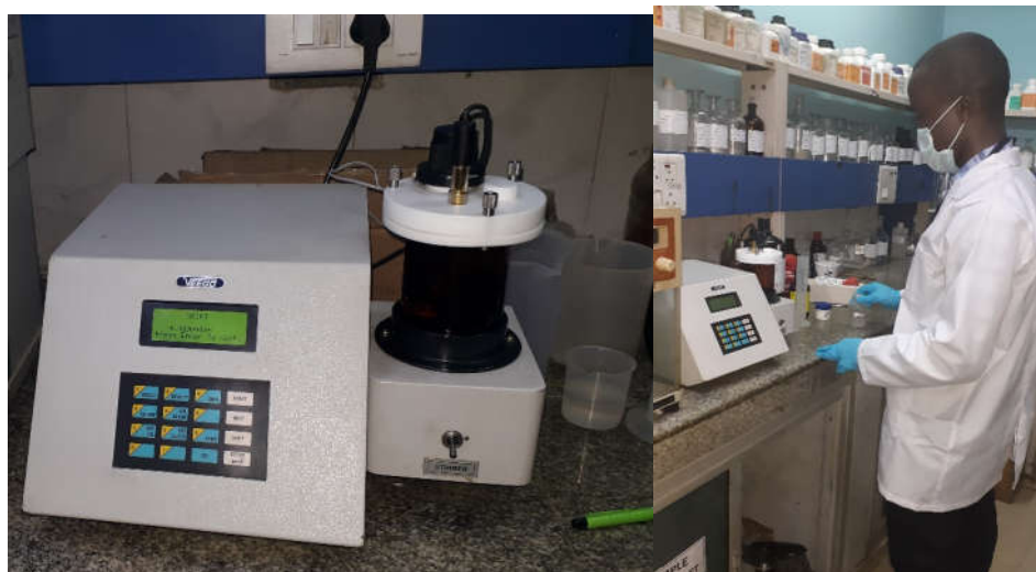
Figure 3.13: Water content determination set up.
