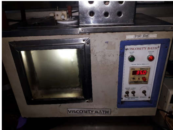
Figure 3.16: Viscosity Measurement Setup Experiment.
