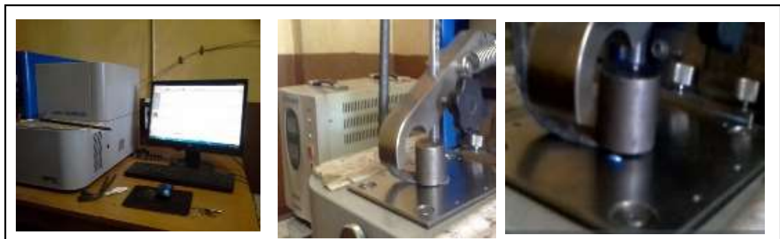
(a) Specromax machine (b) spark stand with specimen (c) ignited spark with specimen
