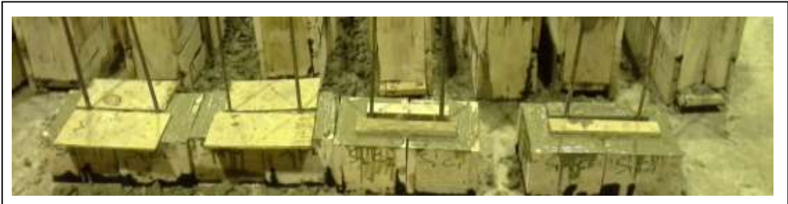
Plate 3.5: Prepared concrete cubes samples with inserted rebar for bond test
