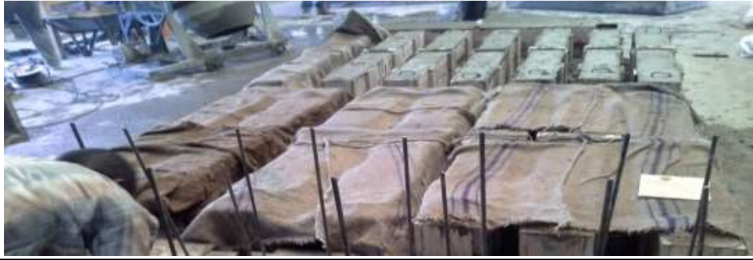
Plate 3.8: Mode of curing for RC beam, concrete cubes and bonding cubes specimens
