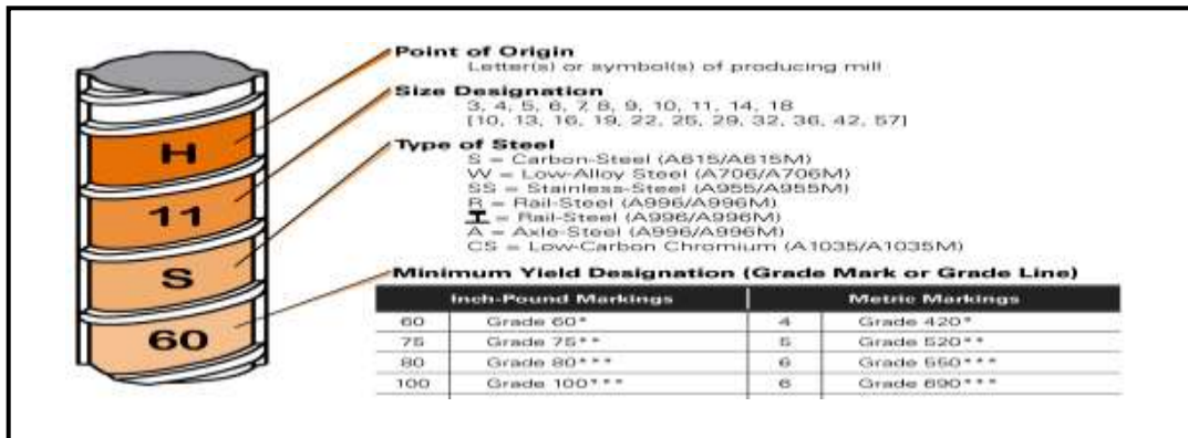
Figure 2.10: Standard rebars' marking sample
