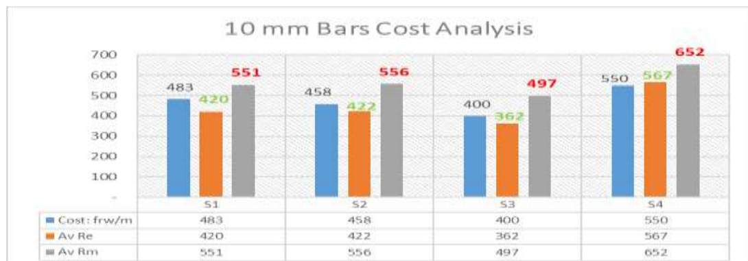
Figure 4.8: Rebars cost comparison: Y10 mm (frw/m)
