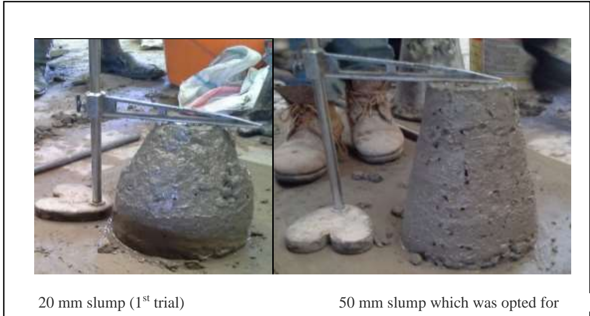
Plate 3.2: Concrete mix trials and measure of plastic concrete slump.
