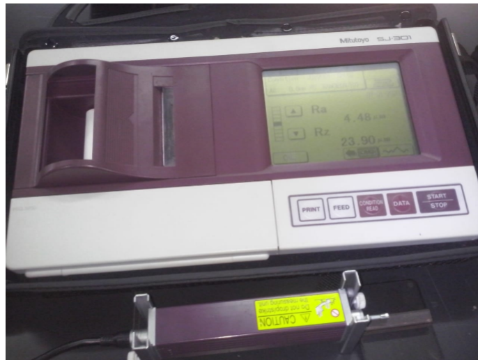
Figure 3.7: Set up for measuring surface roughness using MITUTOYO SJ-30 surface roughness tester
