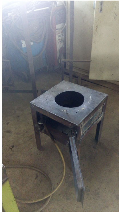
Figure 3.7: Support structure for the reactor
