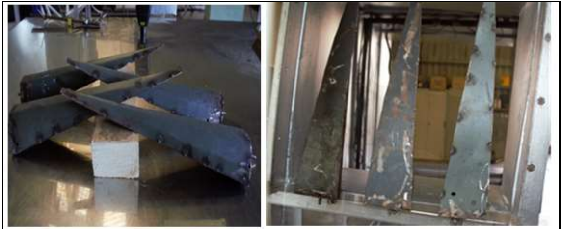
Figure 3.4: Turbulence generating wedge mechanism
