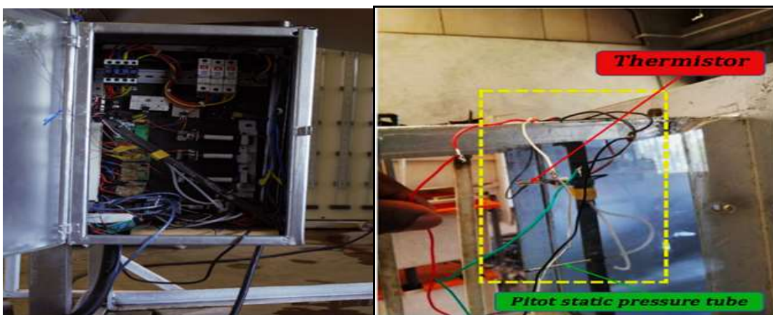
Figure 3.9: Pitot-pressure tube and thermistor measurement assembly
