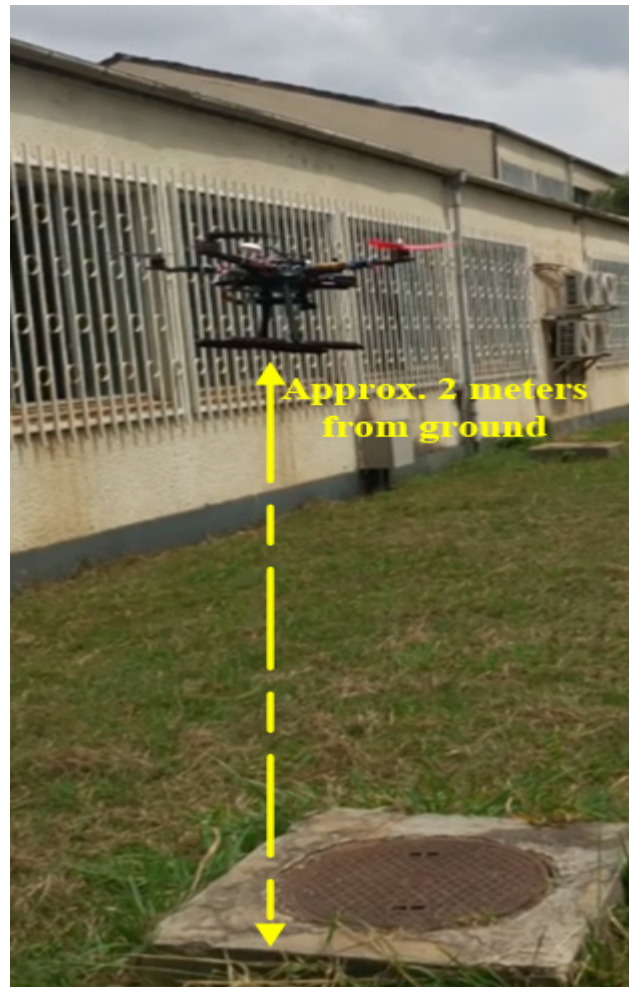
Figure 4.18: Flight hover under rotor fault with the proposed control algorithm
