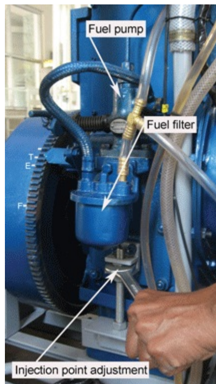
Figure 3.25: Injection timing adjustment system
