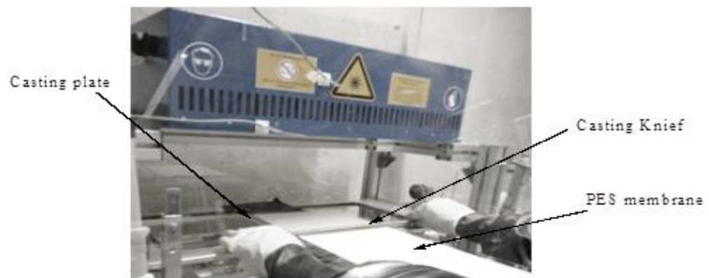
(a) PBM coating process conducted in a casting chamber
