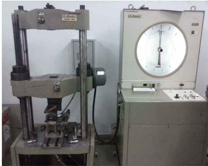
Figure 3.17: Bending testing machine used for experiments
