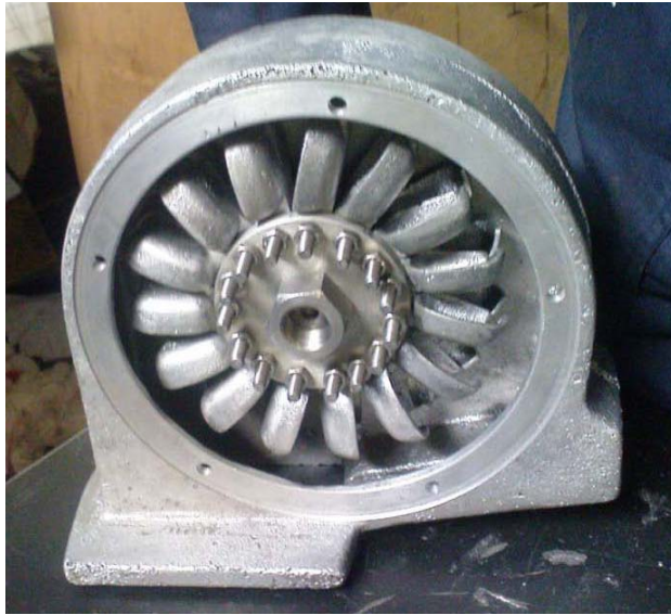
Figure 1: Aluminum Pelton turbine fabricated at JKUAT
