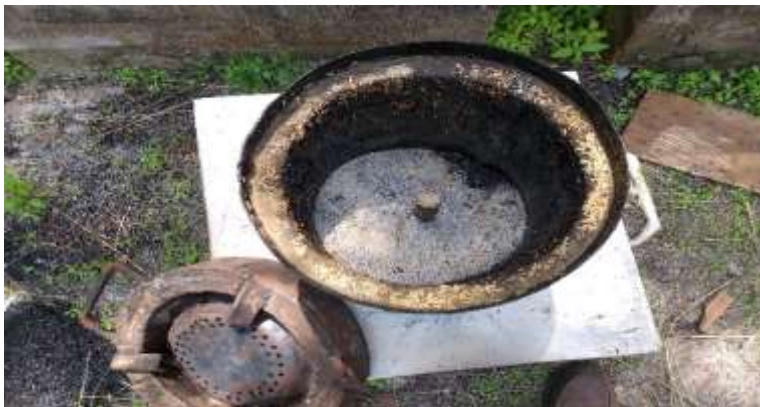
Plate 4.3: Silica extraction oxidation reactor with RHA
