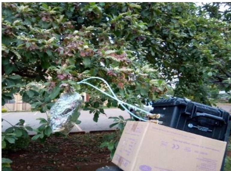
Figure 3. 3: Plant headspace volatile collection using a portable field pump
