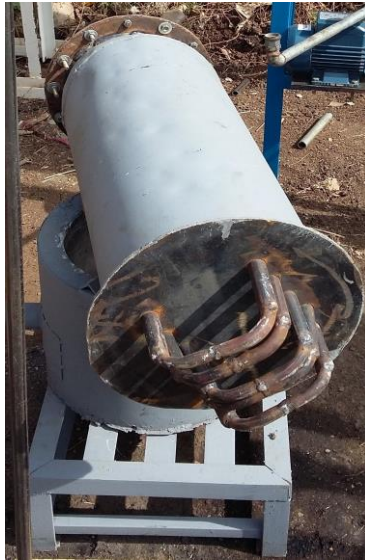
Figure 3.7: The water tubes installed in steam drum
