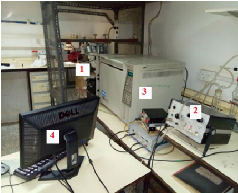
Plate 3.1: Gas Chromatography- Electroantennodetection set up. 1 = antennal mount; 2 = Gas Chromatography – Mass Spectrophometry 3=amplifier; 4= Display computer
