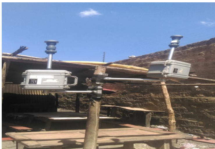
Figure 3:7: MiniVol tactical air sampler on sampling site at industrial area.
