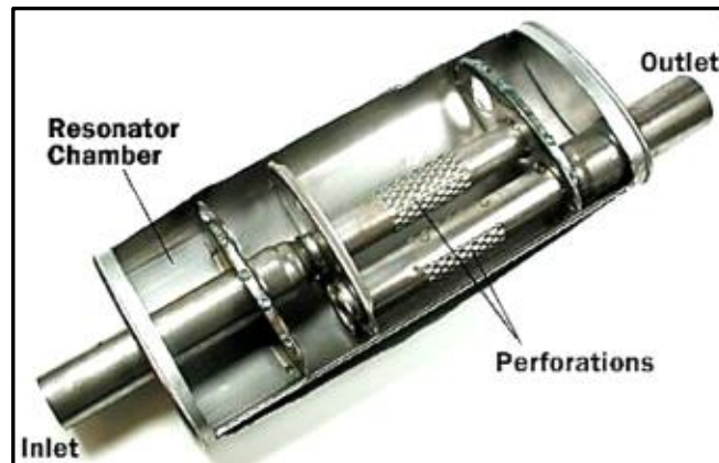
Figure 2.4: Reactive Silencer
