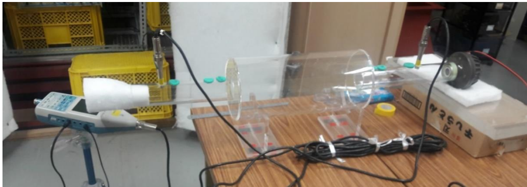
Plate 4.1: Simple Expansion Chamber data collection setup
