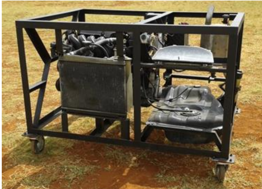
Plate 3.1: A 1,500cc VVT-i gasoline engine noise source and test rig
