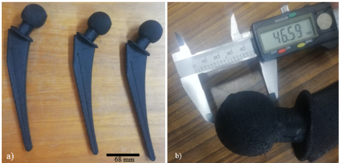
Figure 3.7: (a) 3D printed after the support removal, (b) Measuring of part after 3D printing.
