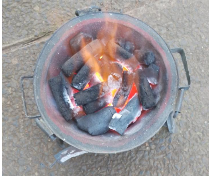
Plate G3: Image of Ignited Charcoal and Briquettes in the Cook Stove
