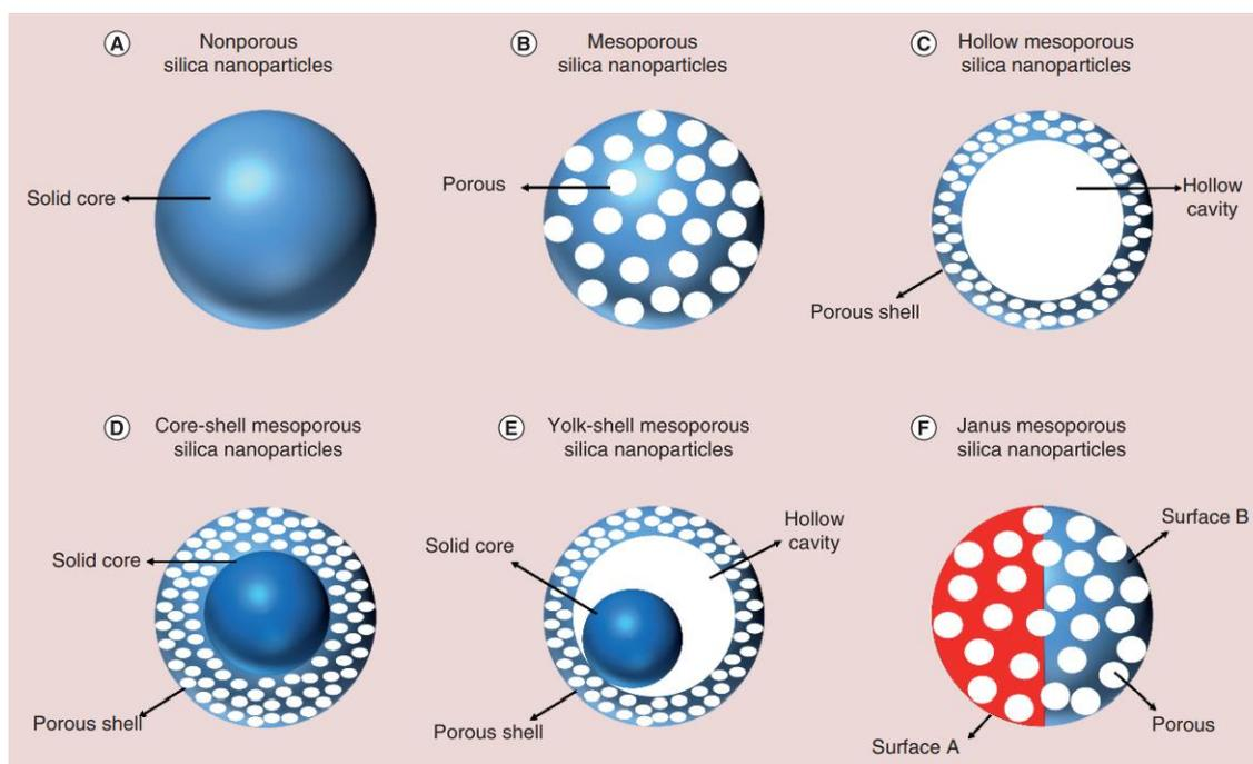
**Figure 2.5: Different types of silica nanoparticles commonly used for biomedical applications.**
