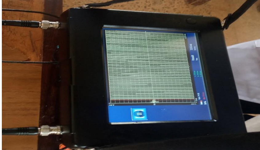
Plate 3.7: Concrete Ultrasonic Pulse Velocity testing equipment
