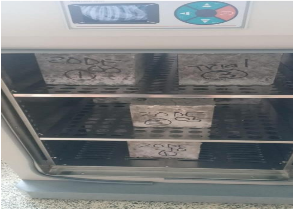
Plate 3.5: Water absorption testing of concrete with SUSFM material
