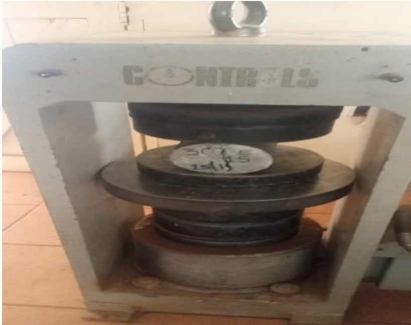
Plate 3.6: Testing of concrete specimens for splitting tensile strength
