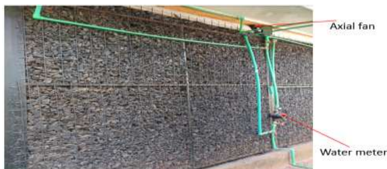
Figure 3.6: External view of the improved evaporative charcoal cooler
