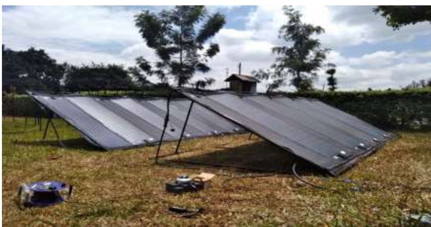
Figure 3.5: Thin-film PV system tilt angle set-up.
