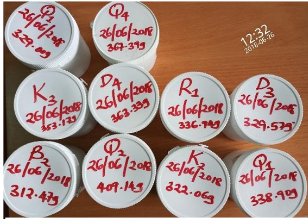
i). Weighed, closed and labelled soil samples to be kept for 30 days
