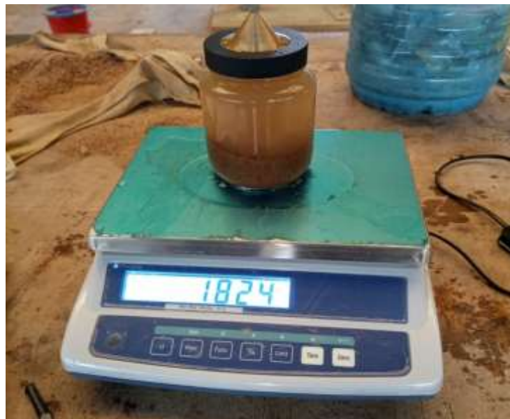
Specific Gravity Test - Pycnometer/ Gas Jar Method
