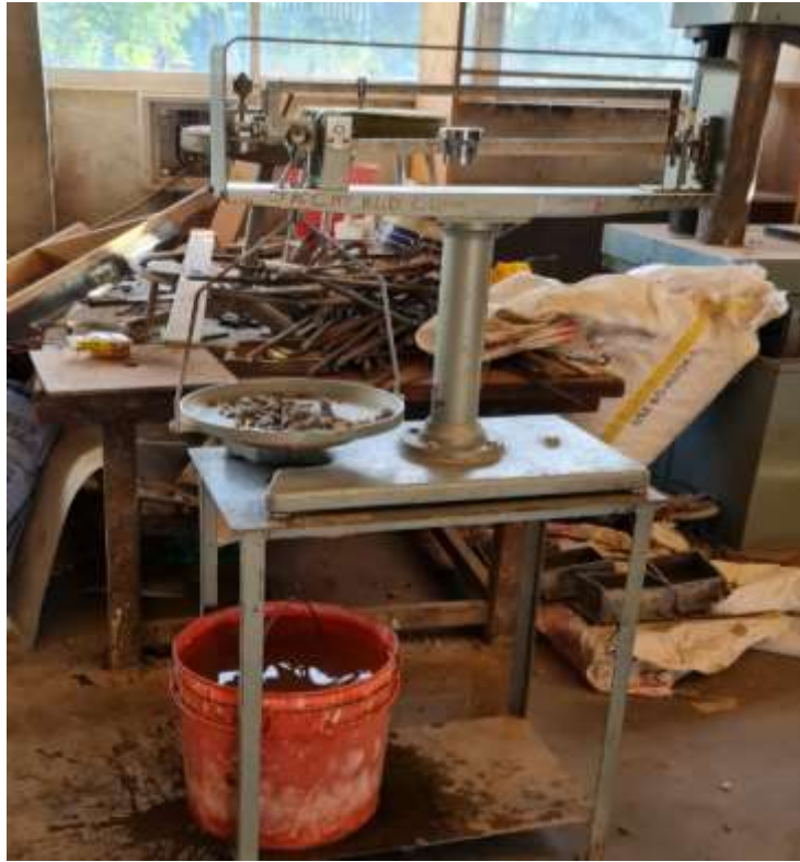
Specific Gravity Test - Wire Basket Method
