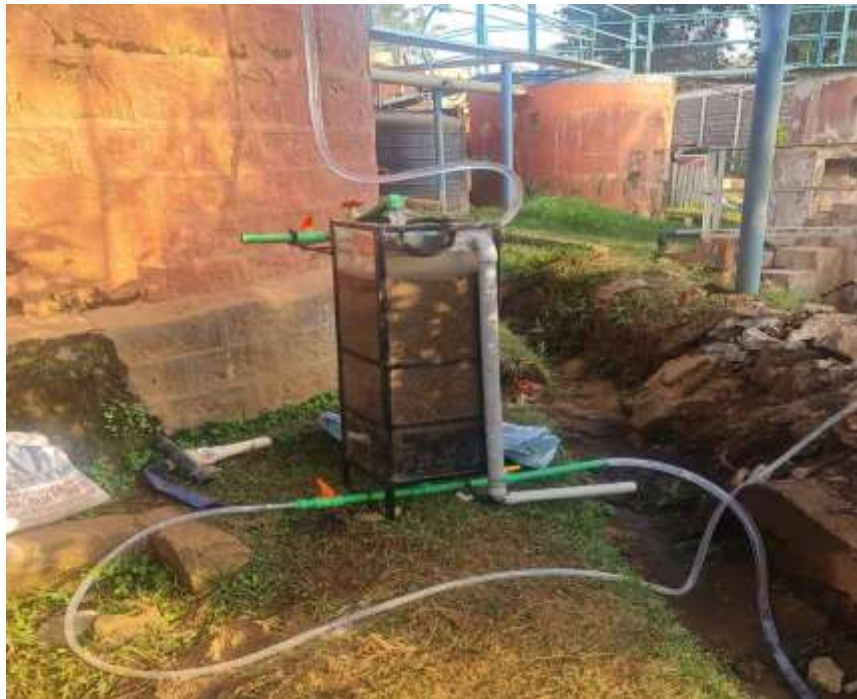
Model Filtration Unit Setup within an Existing Water Treatment Plant
