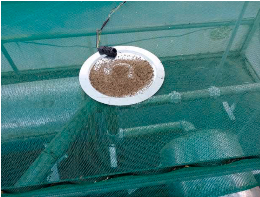
Fig. 4. Thin layer drying of black nightshade seeds on a drying tray.
