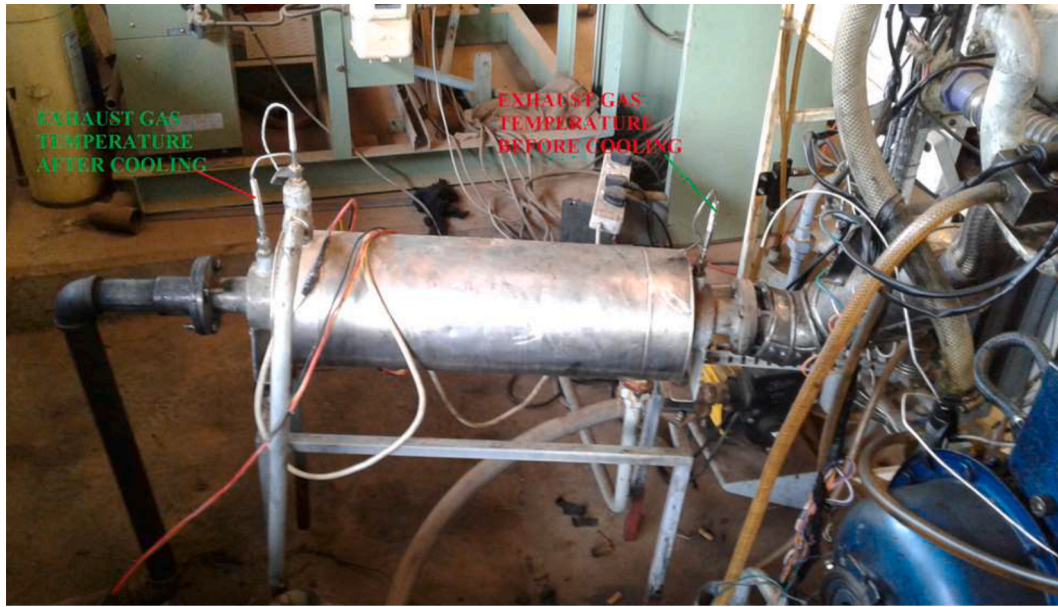
Fig. 6. Location of thermocouple temperature sensors for exhaust gas.
