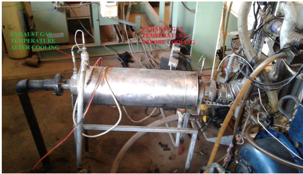
Plate B.7: Location of thermocouple temperature sensors for exhaust gas
