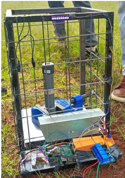
Fig. 16 Static fire test stand assembly with solid rocket motor
