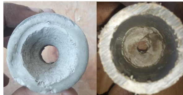
Fig. 14 Fabricated de Laval nozzle (left: diverging side, right: converging side)
