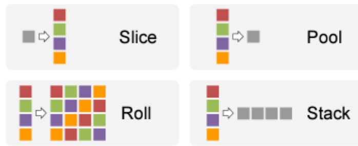
Figure 2.15: The Four Operations that Constitute Framework for Building Rotation Equivariant Neural Networks
