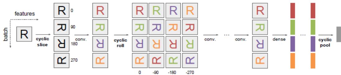
Figure 2.16: Schematic Representation of the Effect of the Cyclic Slice, Roll and Pool Operations on the Feature Maps in a CNN
