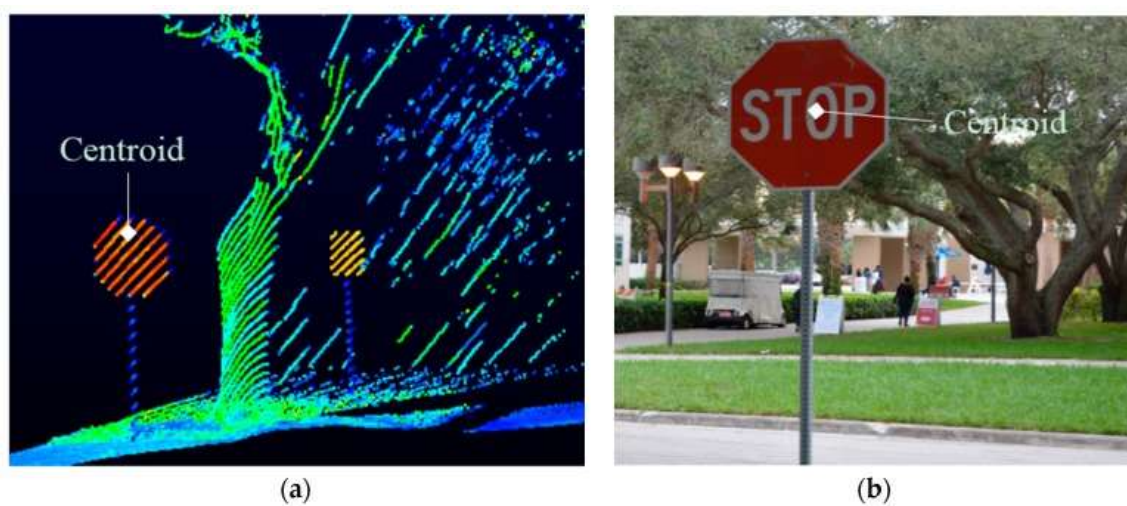
Figure 4.12: Extraction of Road Signs from Lidar Point Clouds and Images
