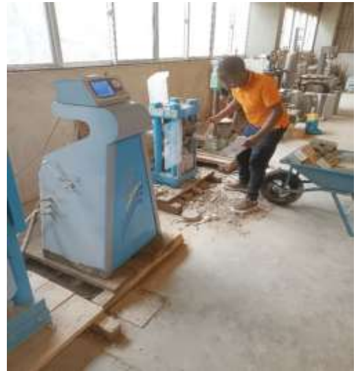
(b) compression strength testing of the blocks
