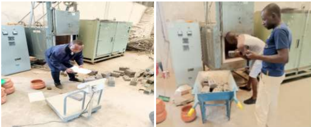
(b) Weighing and loading bricks into the electrical furnace at JKUAT engineering laboratory.
