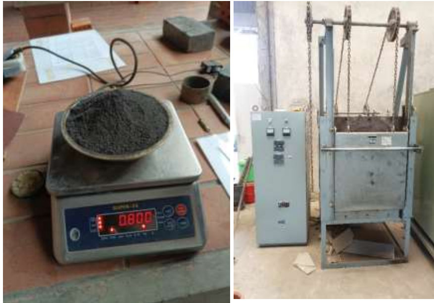
Plate 1: Stabilized clay soil Atterberg limit
