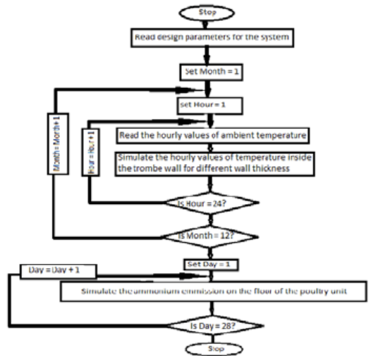
Fig. 2.1: Simulating brooder temperatures and ammonia concentration (source: Authors, 2019)
