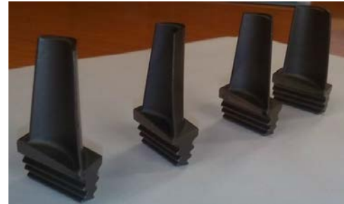
Figure 1: High Pressure (HP), PT6A-114A engine CT blades
