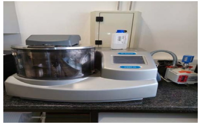
Figure 5: StruersTegramin 30, automatic grinder and polisher
