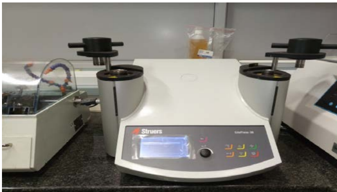
Figure 4: StruersCito Press 30, hot compression mounting machine
