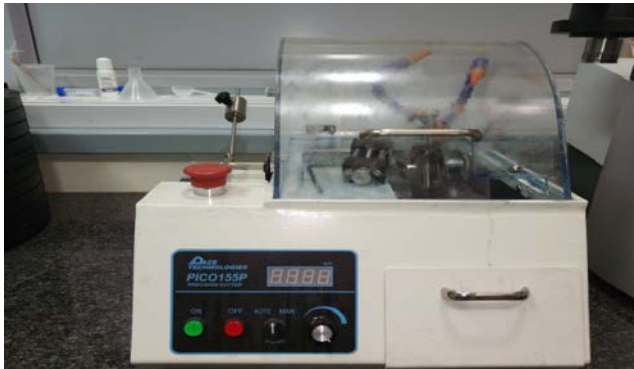
Figure 3: Dace Technologies, Picco 155P, precision cutter
