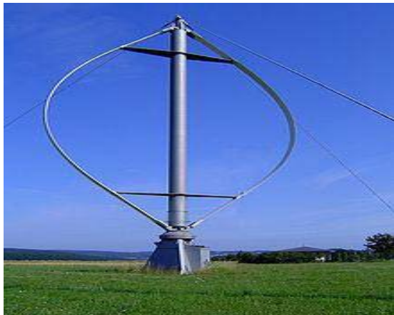
Figure 4: Vertical axis turbine type
