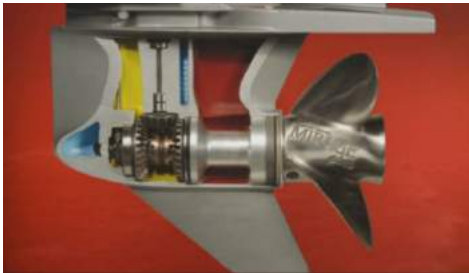
Fig. 3. Propulsion system of an outboard engine [13]
